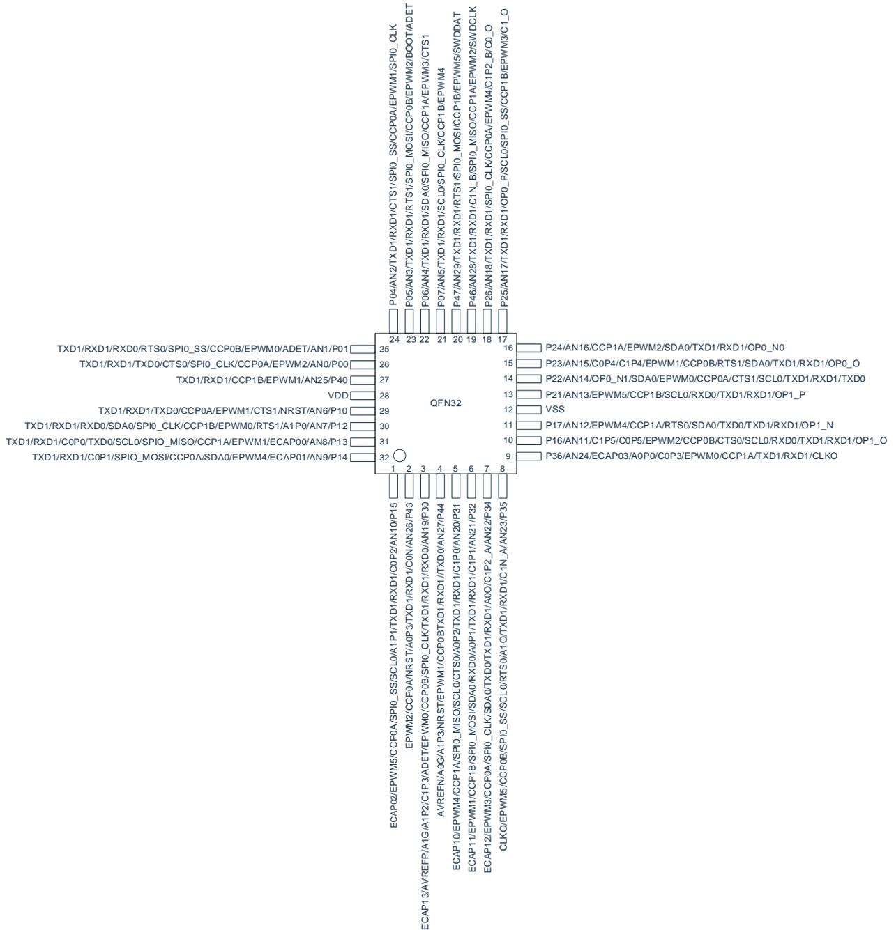
Note: All pins in the pinout diagram can be mapped to TXD1 and RXD1 functions.
